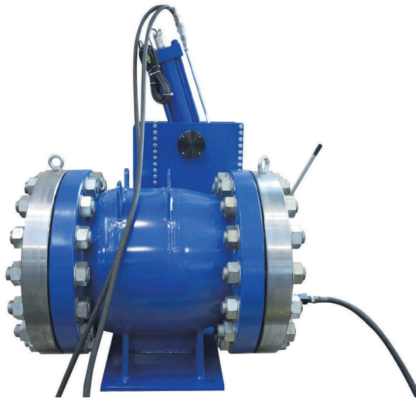
F600 PN100 HYDRAULIC TEST (PRESSURE TEST = 150 BAR)
