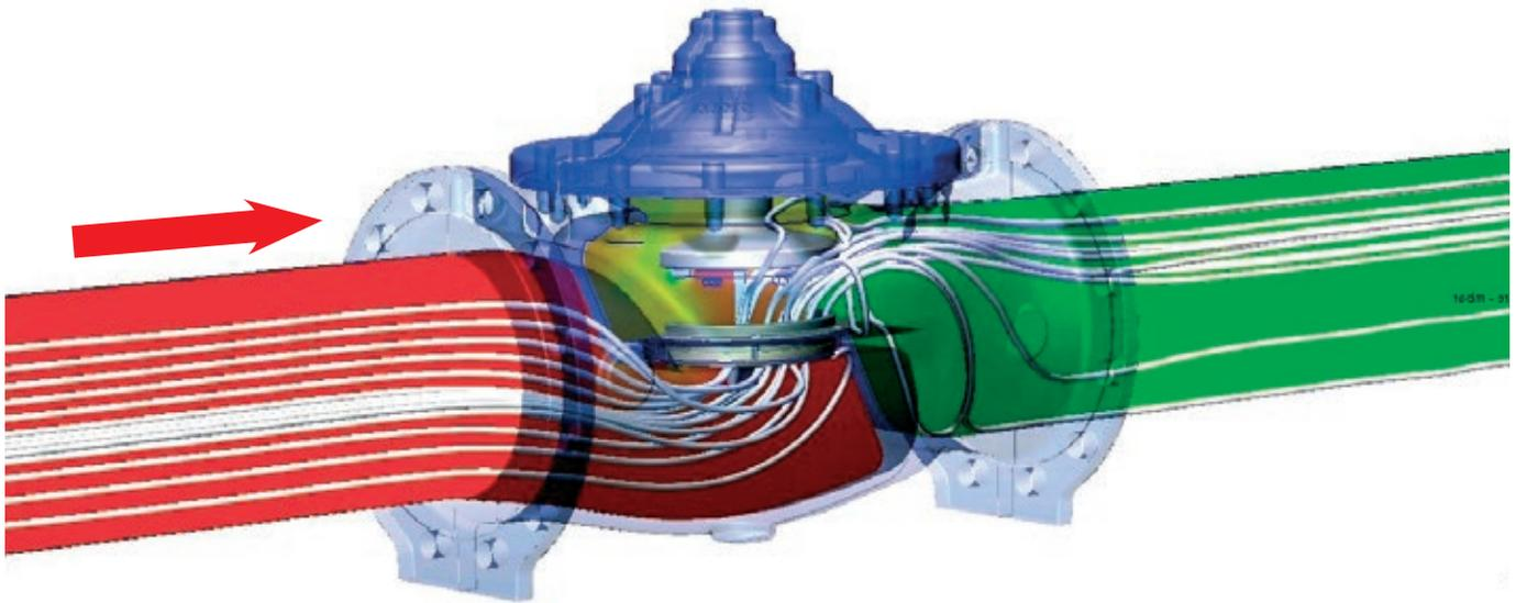
*Automatic control valves, as defined by EN1074-5 standard: "have the integral capacity to control the function using energy from the conveyed water by adjusting the position of the shutter. They can be directly operated, i.e. the force is applied (via a spring or diaphragm) directly to the shutter." Alternatively, "They can be pilot operated i.e. the force is applied through an adjustable pilot valve".*
