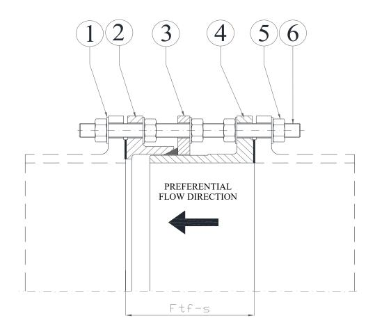
Dismantling joint consist of the following main parts:
