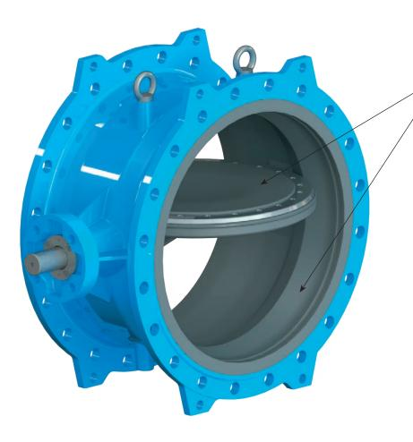
Body and disc surface, in contact with the fluid, is completely lined with a rubber layer which allows additional protection to the corrosion due to brackish waters and significantly increases lifespan of the valve.
