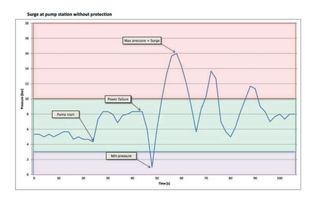
By installing a surge anticipator/pressure relief valve it is possible to reduce strongly the surge effects the system.
