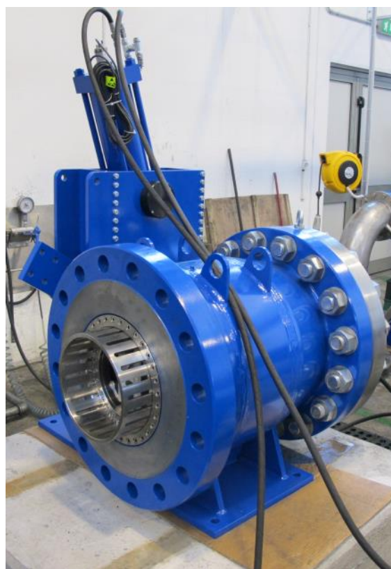
F600 PN100 HYDRAULIC TEST (PRESSURE TEST = 150 BAR)
